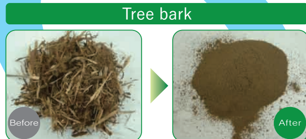
Sample 150g / Stainless steel container 250ml / Stainless steel 20 mm x 12 pieces / Liquid nitrogen
