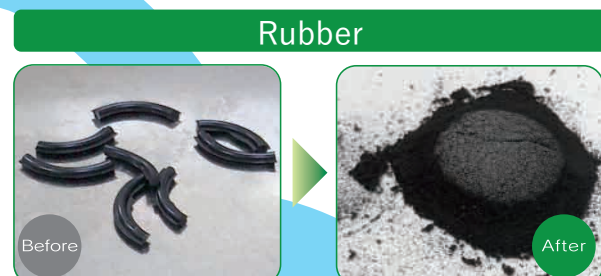
Sample 500mg / 13ml aluminum case / stainless steel 15 mm x 1 / liquid nitrogen
