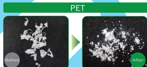
Sample 500mg / 13ml aluminum case / stainless steel 15 mm x 1 / liquid nitrogen
