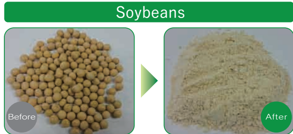
Sample 100g / Stainless steel container 250ml / Stainless steel 20 mm x 12 pieces / Liquid nitrogen
