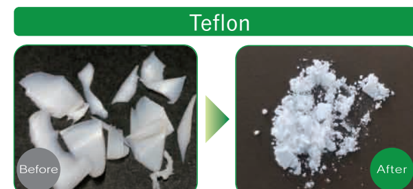
Sample 50g / Stainless steel container 250ml / Stainless steel 20 mm x 12 pieces
